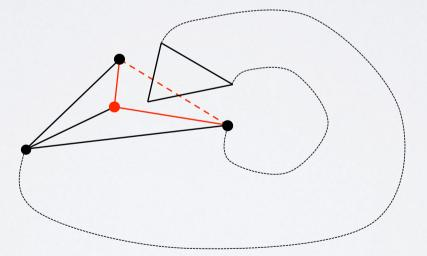
similar problems with edge collapse on concave boundary and vertex split on convex boundary
