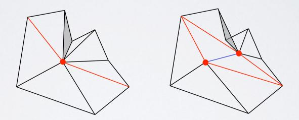
flips can be detected by a local test on the orientation of faces: flips changes orientation from clockwise to counter-clockwise and viceversa
